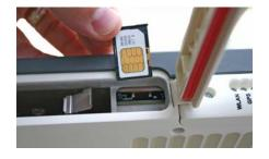
4. Install the USIM/SIM card in the card holder with the gold shield facing up. Snap the card into place in the holder.
