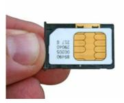
5. With the card in place, orient the holder with the card's gold shield facing down. Place the holder back in its slot in the MT.
