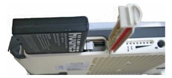
3. Push the button on the left-hand side of the USIM/SIM card holder. This releases the holder from its slot.
