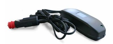
The DC power adaptor (HNS P/N 3004065-0001) can be purchased through Hughes Network Systems. It has an operating temperature range of -25°C to +55°C and provides an output voltage of 20 VDC. It can be used with input voltages in the range 10 to 32VDC.
