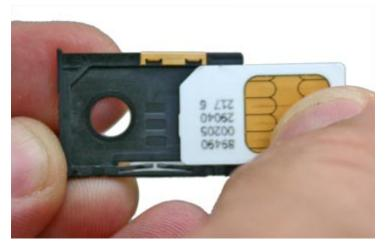
5. With the card in place, orient the holder with the card's gold contacts facing down. Place the holder back in its slot in the BGAN terminal.
