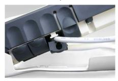
2. At the Terminal connection point, slide the cable through the rubber door slot in order to secure and protect the connection.
