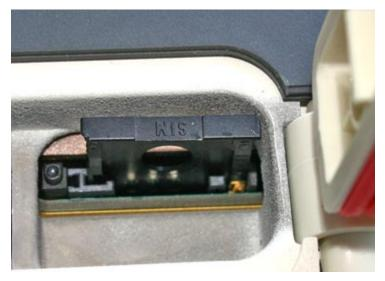
4. Install the USIM/SIM card in the card holder making sure it is snapped into place.
